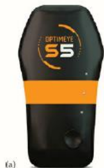
Figure 1.6 (a) A GPS receiver used to track player motion. (b) The receiver is housed in a vest worn by the player.
